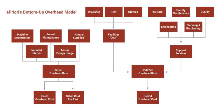
\*By default aPriori accounts for facilities cost in Indirect Overhead; a digital factory level switch is available to account for in facilities cost in Direct Overhead
