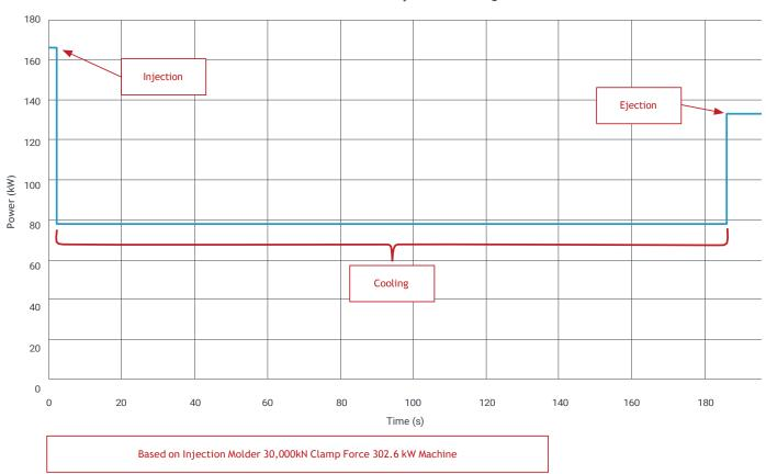
This graphic shows energy used throughout one injection mold cycle. The machine uses high energy as the molten polymer is forced into the mold; then the energy level drops during the cooling phase. Next the mold is pulled apart, which triggers the release of the cooled/solidified part at the same time. This movement uses more energy and so it goes up again. There is always energy used as the plastic is heated and then forced into the mold.
